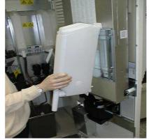
After loading, refit the canister and reopen the closure of the slide.
