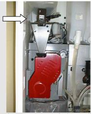
2) The electromagnet of the coffee throw dispensing unit is activated and the canister is open. The correct quantity of ground coffee flows by gravity in the brewer of the espresso coffee group; \*
