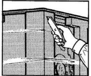
1) Cut the protection film along one of the protection angle bar around the machine
