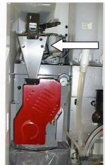
3) The coffee grinder is activated until the preset quantity in the throw dispensing unit is restored;
