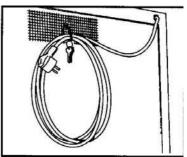
3) Take the key on the rear of the machine, near the power supply cord.
