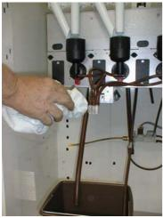
1) With a damp cloth, clean the visible components in the ingredients vend area.
