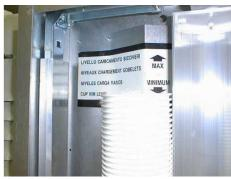
pull the two mobile sides towards The edge of the upper cup of each until they are stack must reach a height between limits indicated on the the sticker of instructions placed inside in the cup feeder. This allows a regular operation of the inside mechanisms of the cup feeder itself:
