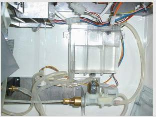
5) The water coming from a water refilling container, in which the water level is kept constant, is conveyed by pressure in the coffee boiler by means of a pump. After the activation of a solenoid valve, the same quantity of warmed up water is then conveyed to the coffee group.
