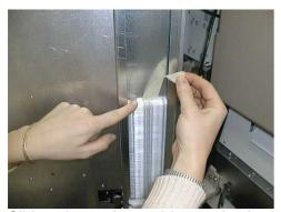
Slide along the guide track the stirrers still hold together with the packing band and, once they have reached the end of the guide, rip the band off.
