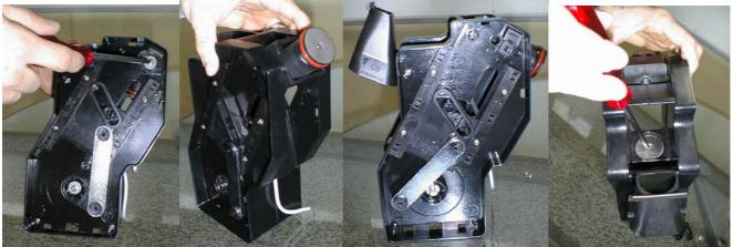
Remove the plates of the superior filter
