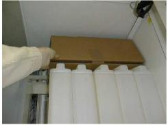
Remove the board prism positioned between the canisters of the ingredients and the top of the cabinet.
