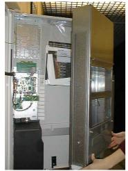
Slide the stirrers still hold together with the packing band along the guide track and, once they have reached the end of the guide, rip the band off.
