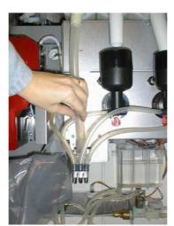
Remove the silicone beverage outlet tubes and pertaining supports. Immerse all parts in the solution.
