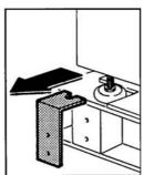
2) Remove the pallet from the machine by lifting the two lateral hooks:
