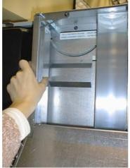
outside. blocked; slide the stacks of cups the towards the inside of machine. keeping them vertical position.
