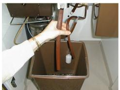
Place the liquid waste disposal bucket on the bottom of the machine, sliding it in the appropriate guide tracks, and insert the drain pipes and the pressure relief tube. Open the tap of the water circuit.
