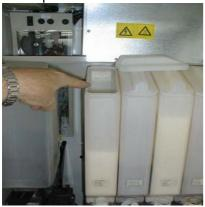
The canisters for instant ingredients can be removed from the machine for an easier loading. Turn the closure of the slide in order to prevent spilling of powder.
